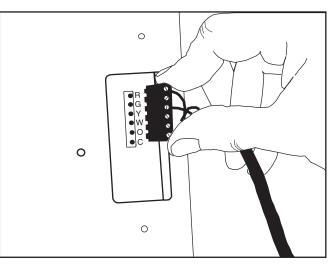
FIGURE 12 — TERMINAL CONNECTOR REMOVAL AND REPLACEMENT
